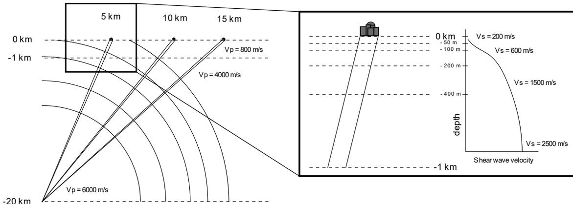
Figure 3. Illustration of an earthquake with the shear wave velocity profile.
