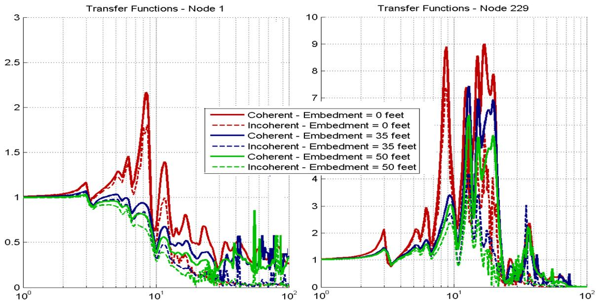
Figure 4. Embedment and Motion Incoherency Effects on Acceleration Transfer Function (ATF) Amplitudes at Basemat Center (Node 1) and at the Top of CIS (Node 229)
