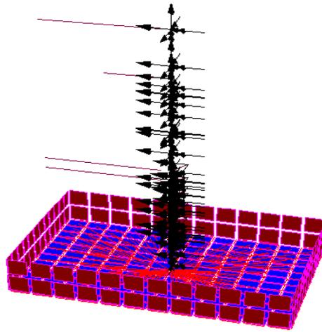
Figure 2 Embedded AP1000-based Stick Model
