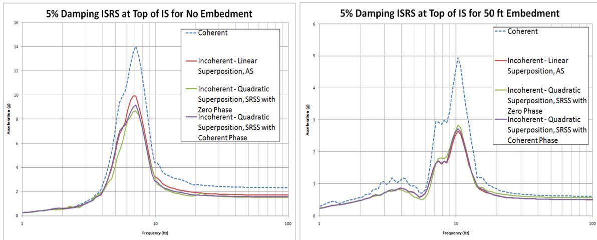
Figure 3 Embedment Effects on the Coherent and Incoherent ISRS Computed at Top of RB Structure
