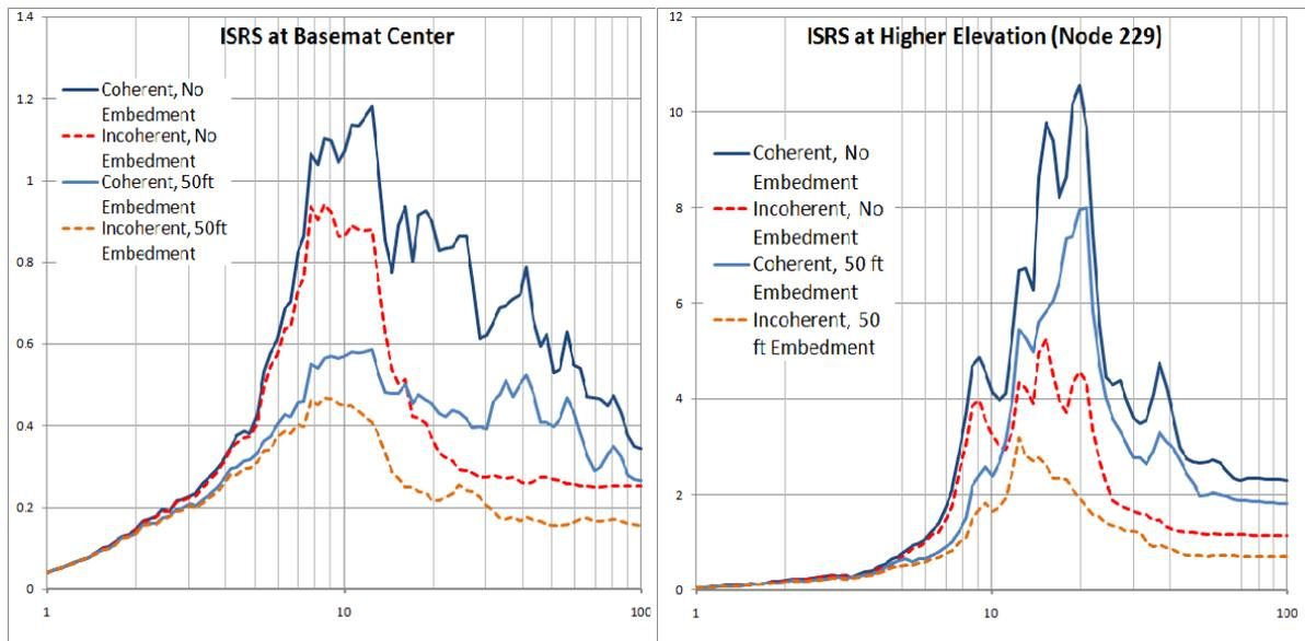
Figure 5 Embedment and Motion Incoherency Effects on 5% Damping ISRS at Basemat Center (Node 1) and at the Top of CIS (Node 229)
