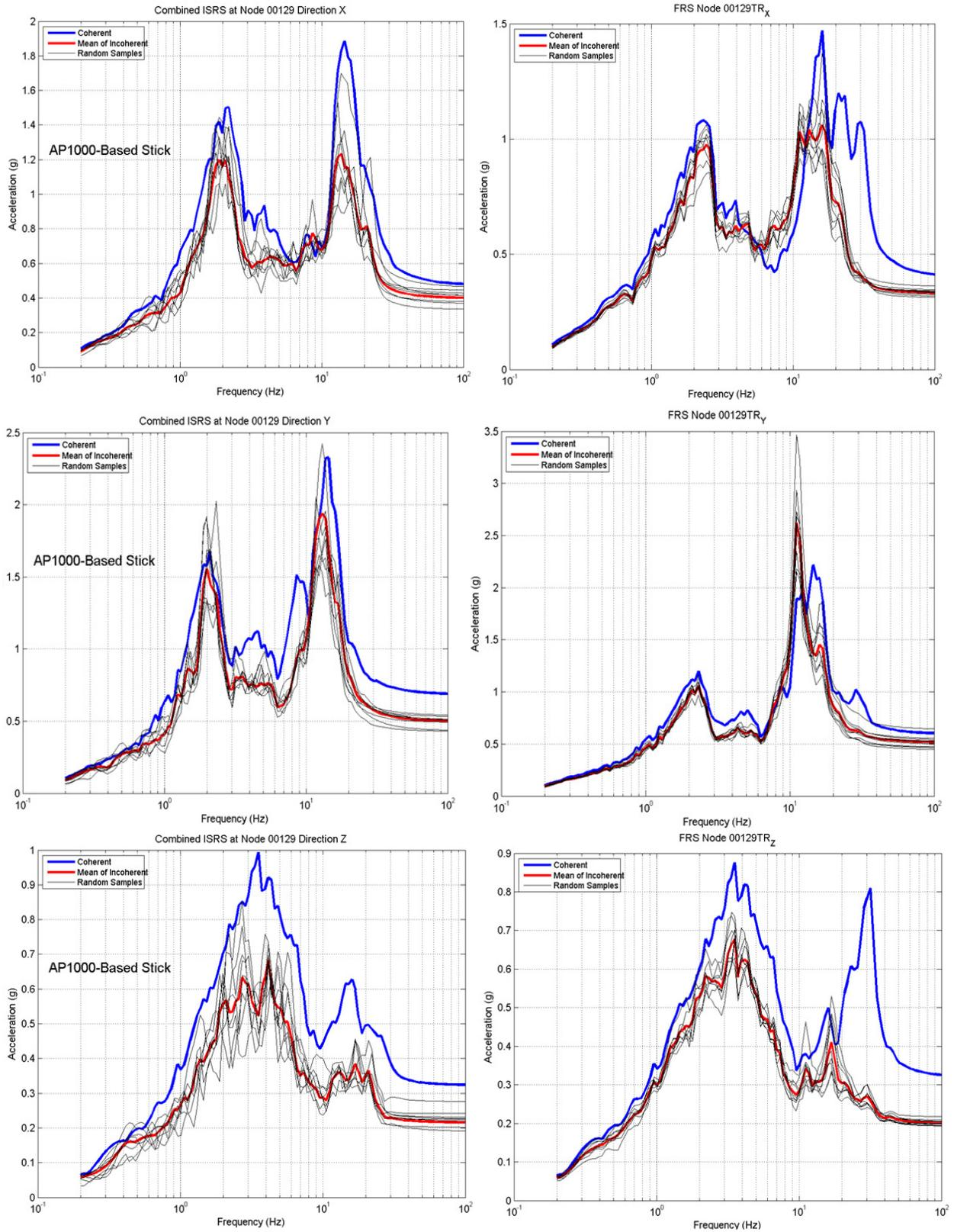
Figure 7 Motion Incoherency Effects for Non-Embedded (left plots) and 40ft Embedded (right plots) AP1000-based Stick on 5% Damping ISRS at Top of CIS for the Soft Soil Conditions (Vs of 1000fps) with the RG 1.60 Seismic Input for X (top), Y(center) and Z (bottom) Directions
