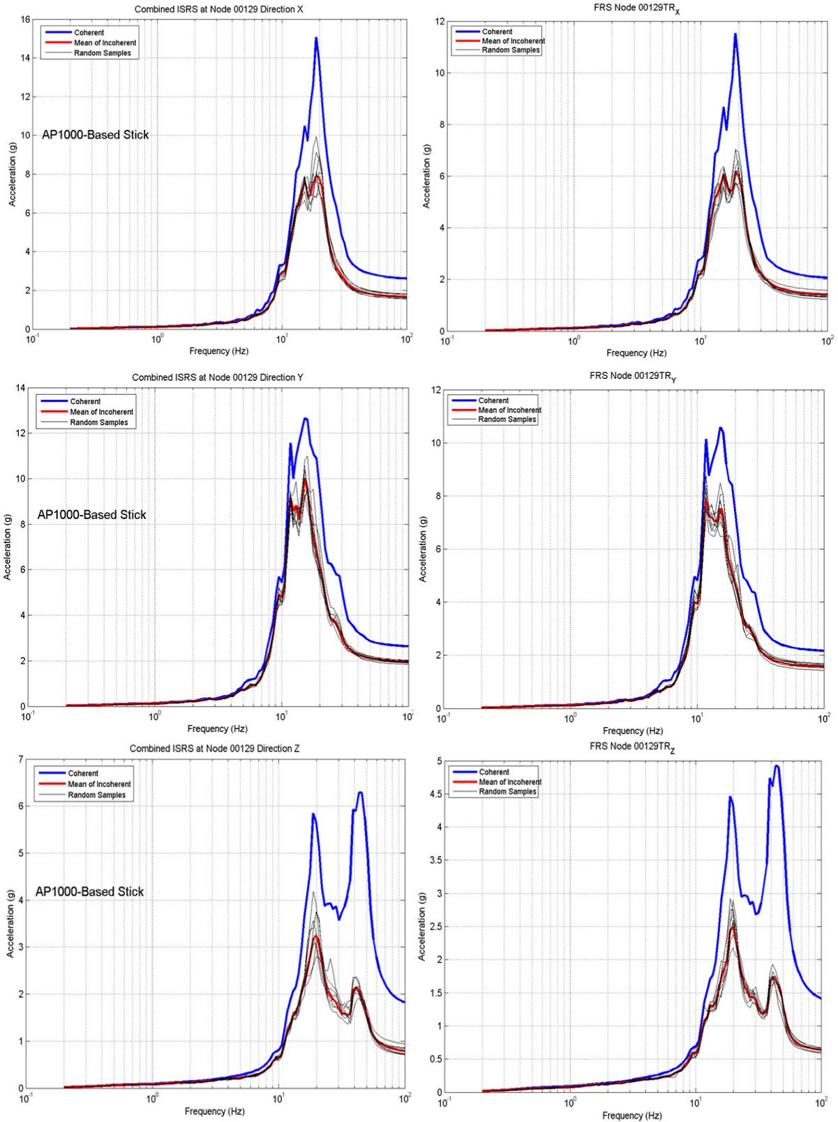
Figure 6 Motion Incoherency Effects for Non-Embedded (left plots) and 40ft Embedded (right plots) AP1000-based Stick on 5% Damping ISRS at Top of CIS for the Hard-Rock Conditions (Vs of 9000fps) with the Hard-Rock Seismic Input for X (top), Y(center) and Z (bottom) Directions.
