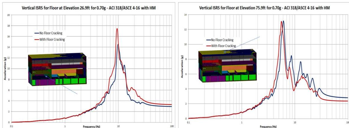
Figure 23 Effects of Floor Cracking on Vertical ISRS for 3<sup>rd</sup> Floor and 6<sup>th</sup> Floor (Roof) Slabs
