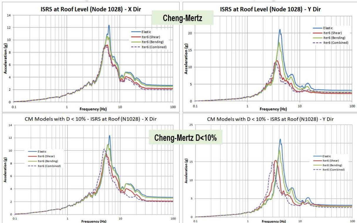
Figure 15 Effects of Equivalent Damping Limitation to 10% Per ASCE 4-16 for Response Level 3
