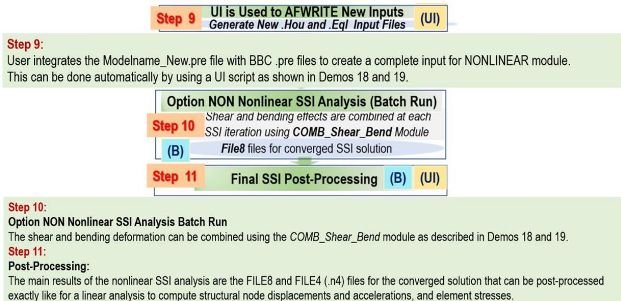
Figure 14 Preparing Inputs (Step 9) and Running Iterative Nonlinear Structure Analysis (Step 10), Plus Post-Processing SSI Nonlinear Responses After Convergence is Reached (Step 11)
