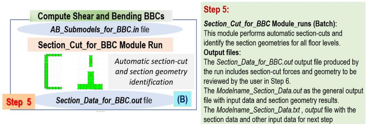
Figure 7 Compute Sectional Forces and Identify Sectional Geometries (Step 5); Details are on right
