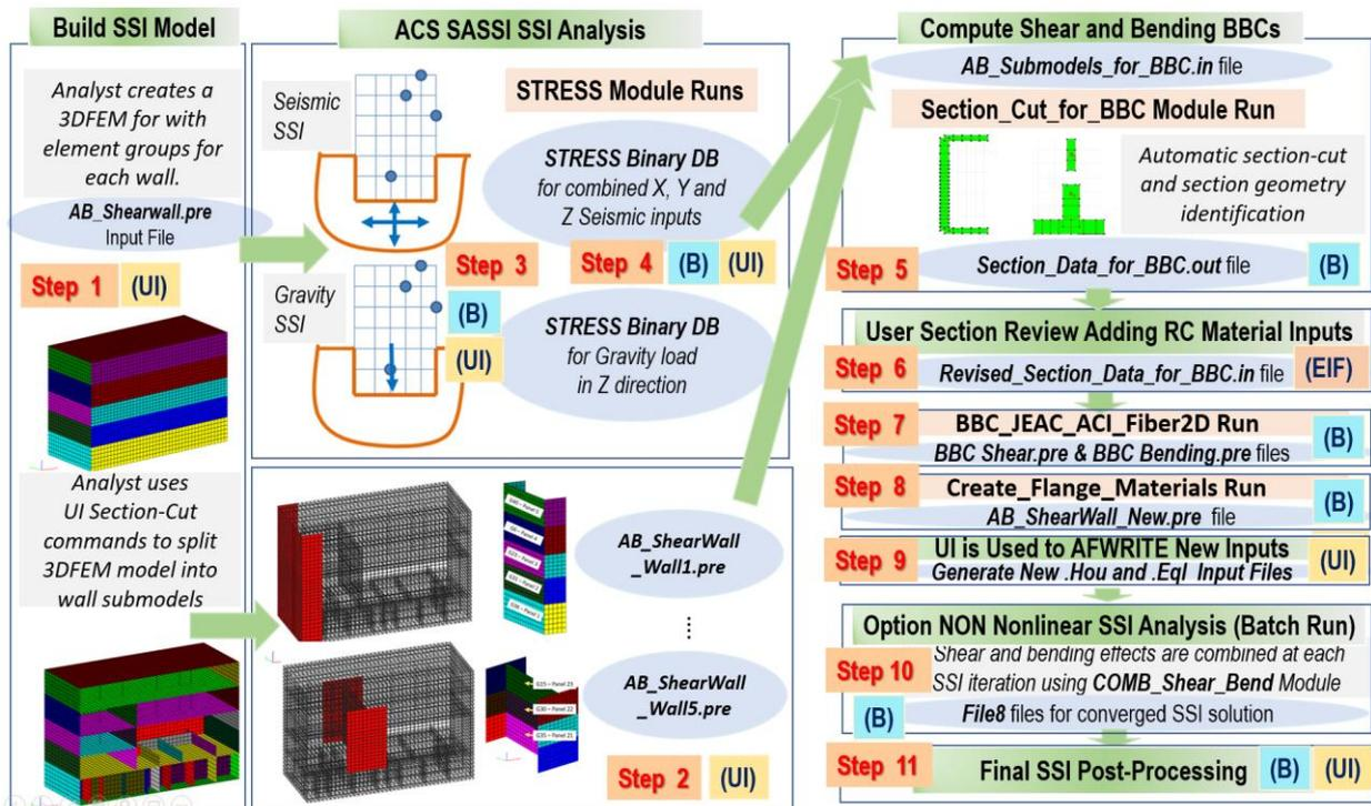
Figure 1 ACS SASSI Option NON Iterative SSI Analysis Flowchart
