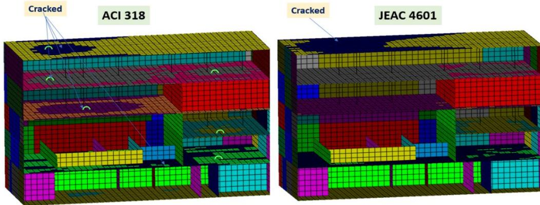
Figure 22 Computed Floor Cracking Patterns Based on US and Japan Standards
