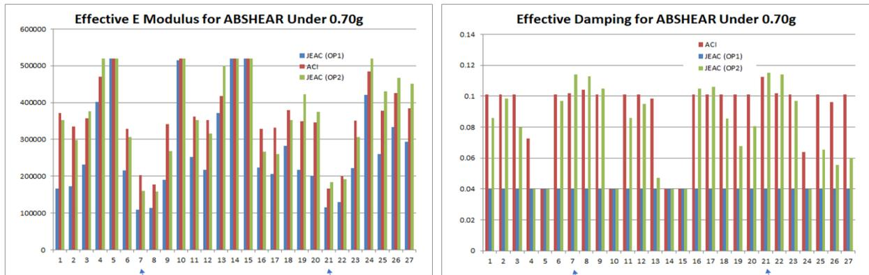
Figure 16 Equivalent Elastic Modulus and Equivalent Damping Due to Shear Effects
