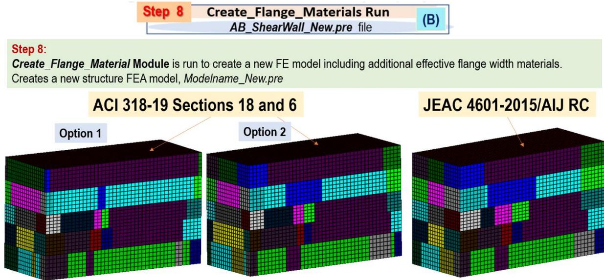
Figure 13 New FE Models Including Nonlinear Flange Materials Using US and Japan Standards
