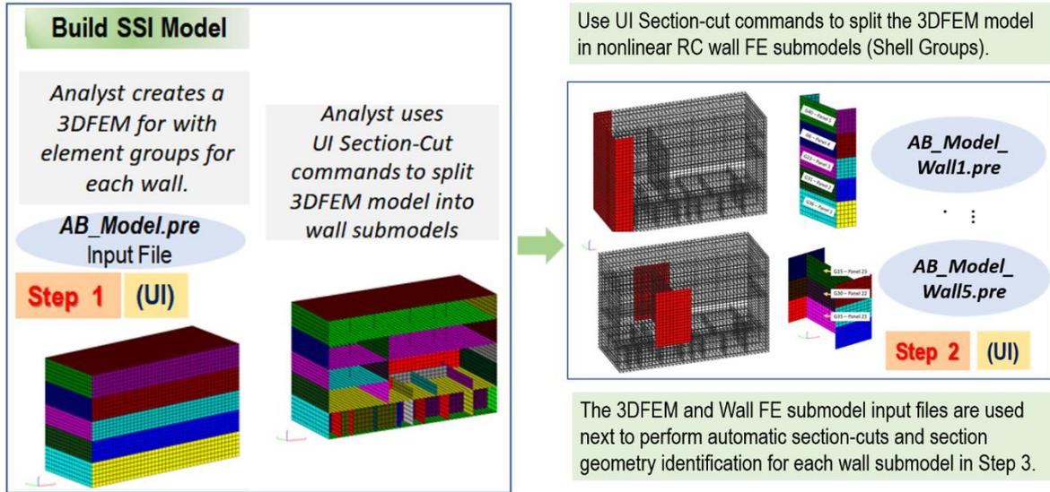
Figure 4 Creating AB SSI Model (Step 1) and RC Wall Submodels (Step 2)
