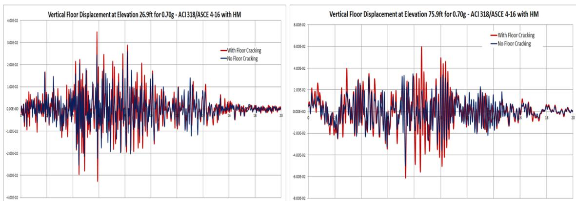
Figure 24 Effects of Floor Cracking on Vertical Displacement for 3<sup>rd</sup> Floor and 6<sup>th</sup> Floor (Roof) Slabs
