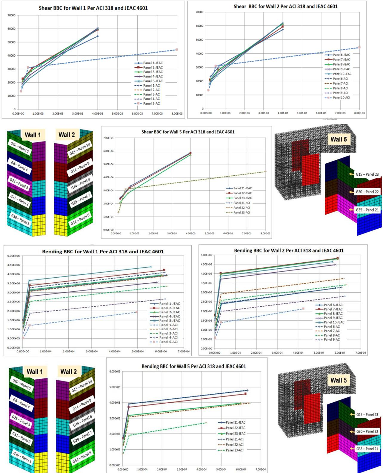
Figure 12 Computed Shear and Bending BBCs for Walls 1, 2 and 5 Based on US and Japan Standards
