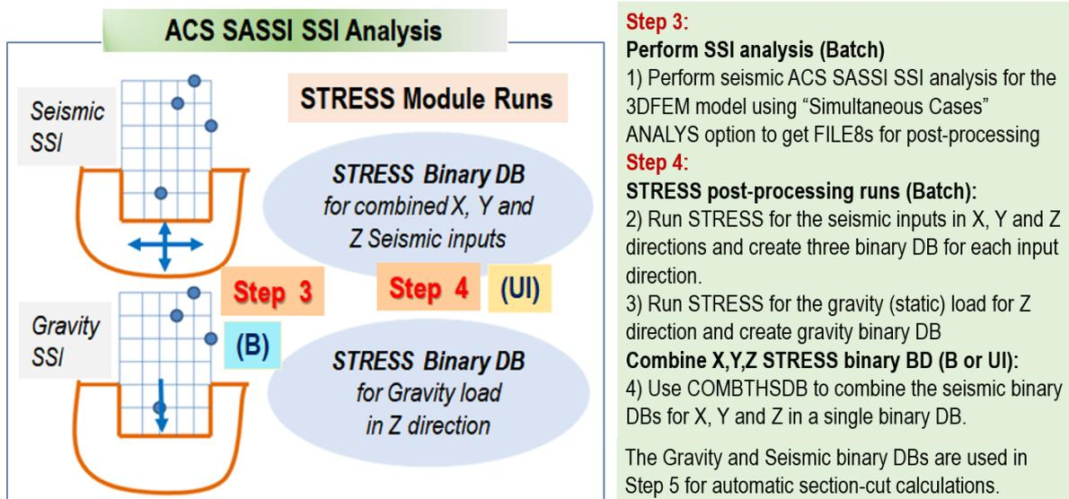
Figure 6 Run SSI Analyses (Step 3) and Compute Structural Stresses (Step 4); Details are on right
