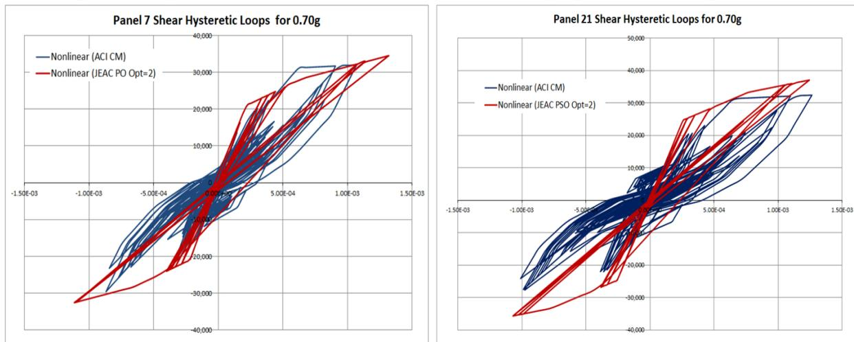
Figure 18 Shear Hysteretic Responses for Wall Panels 7 and 21 (see Figure 12 for locations and BBC)
