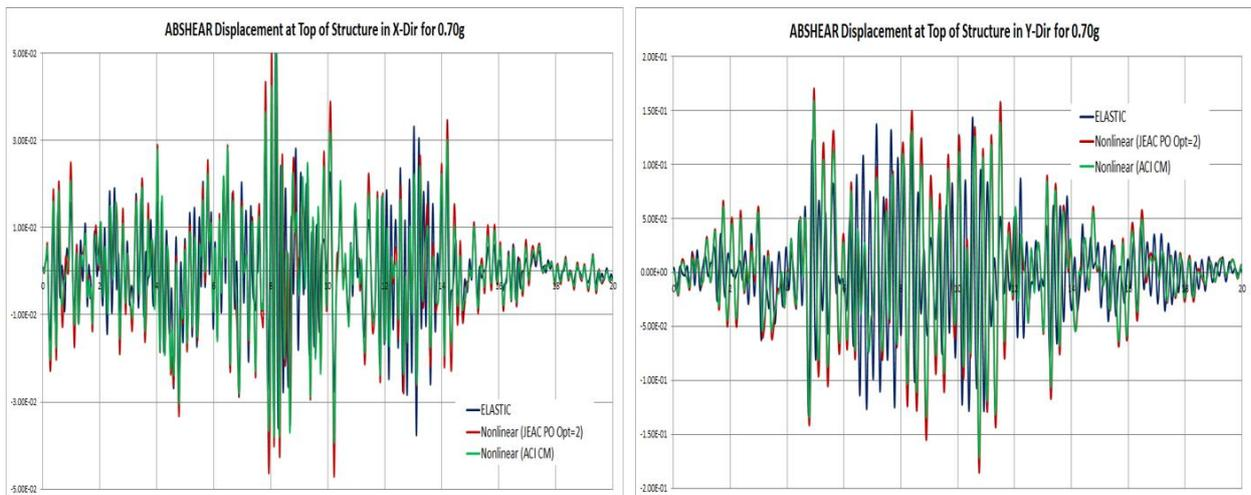
Figure 21 Nonlinear SSI Displacements at Top of AB Structure in X (Long) and Y (Trans) Directions
