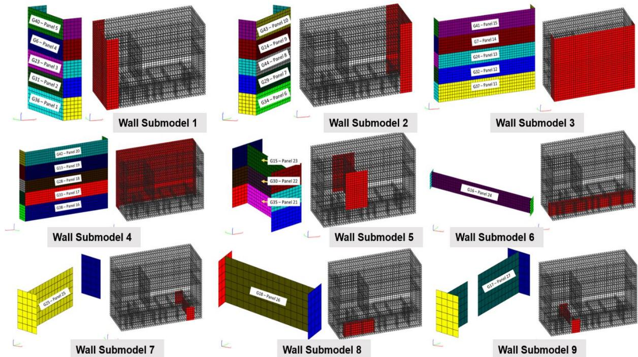
Figure 5 AB Structure Nonlinear RC Wall Submodels (Step 2)
