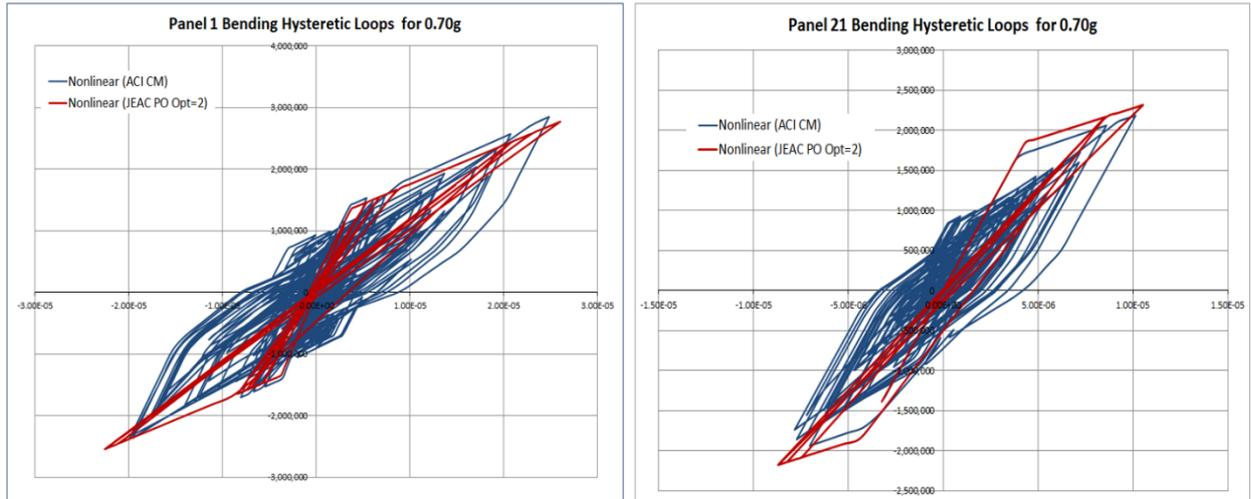
Figure 19 Bending Hysteretic Responses for Panels 7 and 21 (see Figure 12 for locations and BBC)
