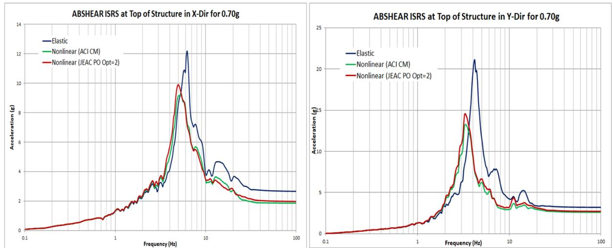
Figure 20 Comparative Nonlinear ISRS at Top of AB Structure in X (Long) and Y (Trans) Directions
