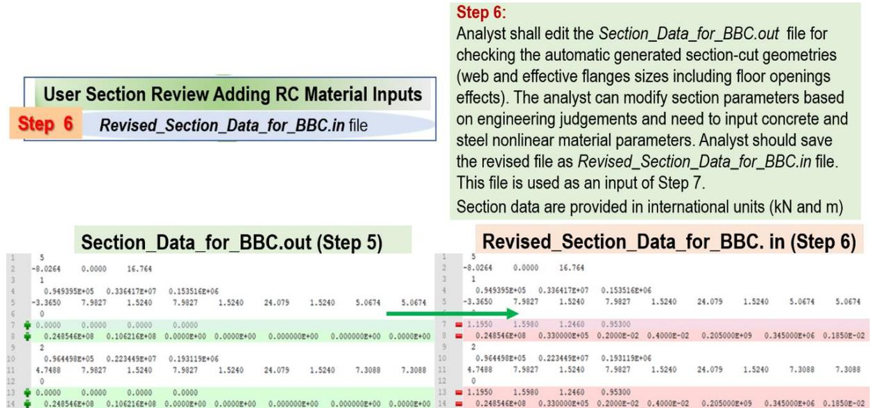
Figure 8 Analyst Reviews Wall Section Forces and Geometry Information (Step 6)
