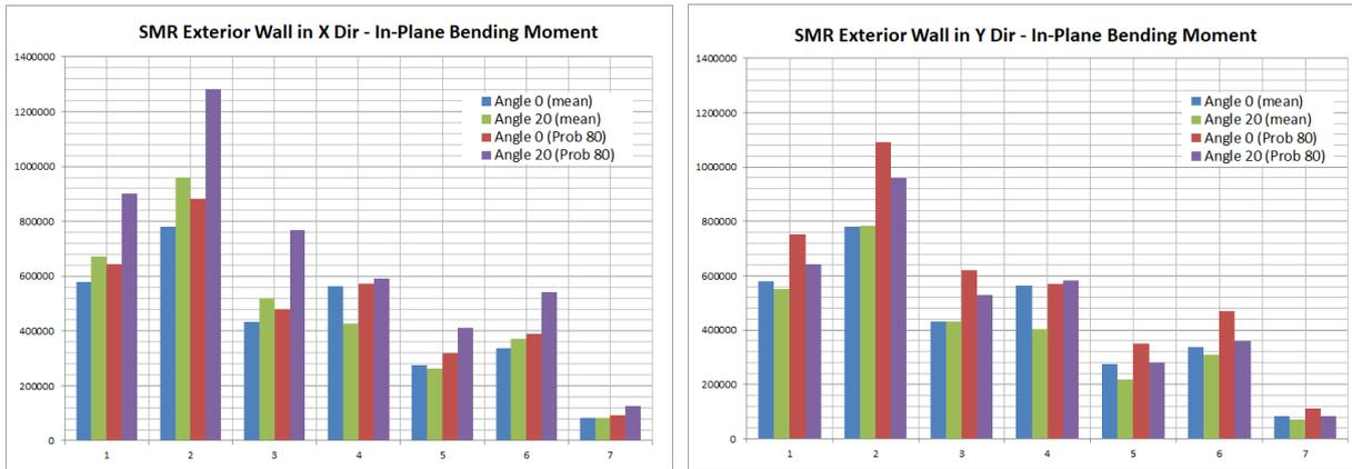
Figure 11 Site 2 Bending Moments in SMR Exterior Walls (for 7 Floor Levels) in X and Y Directions
