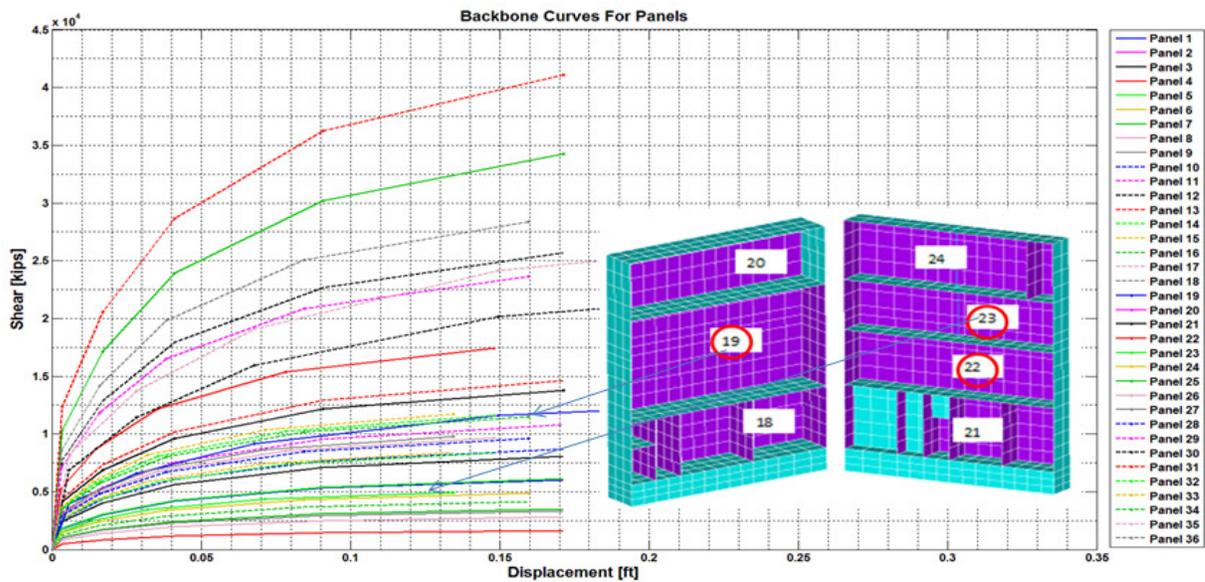
Figure 7 Back-Bone Curves for All 36 Shearwall Panels.
