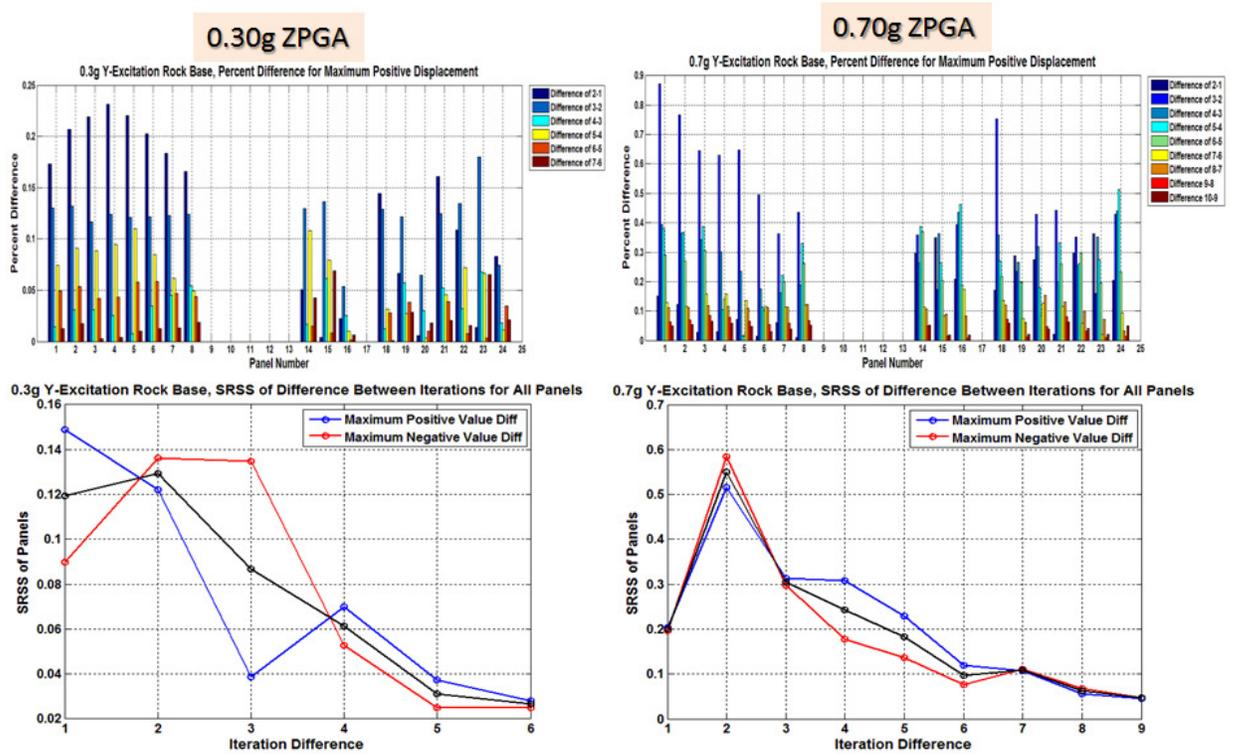
Figure 8 Nonlinear SSI Analysis Convergence for 0.30g and 0.70g Seismic Inputs;
