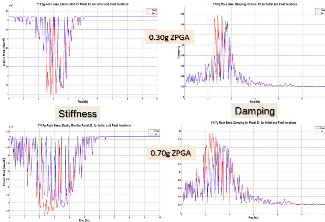
Figure 11 Frequency-Dependent Stiffness and Damping for 0.30g and 0.70g (1<sup>st</sup> and last iterations)
