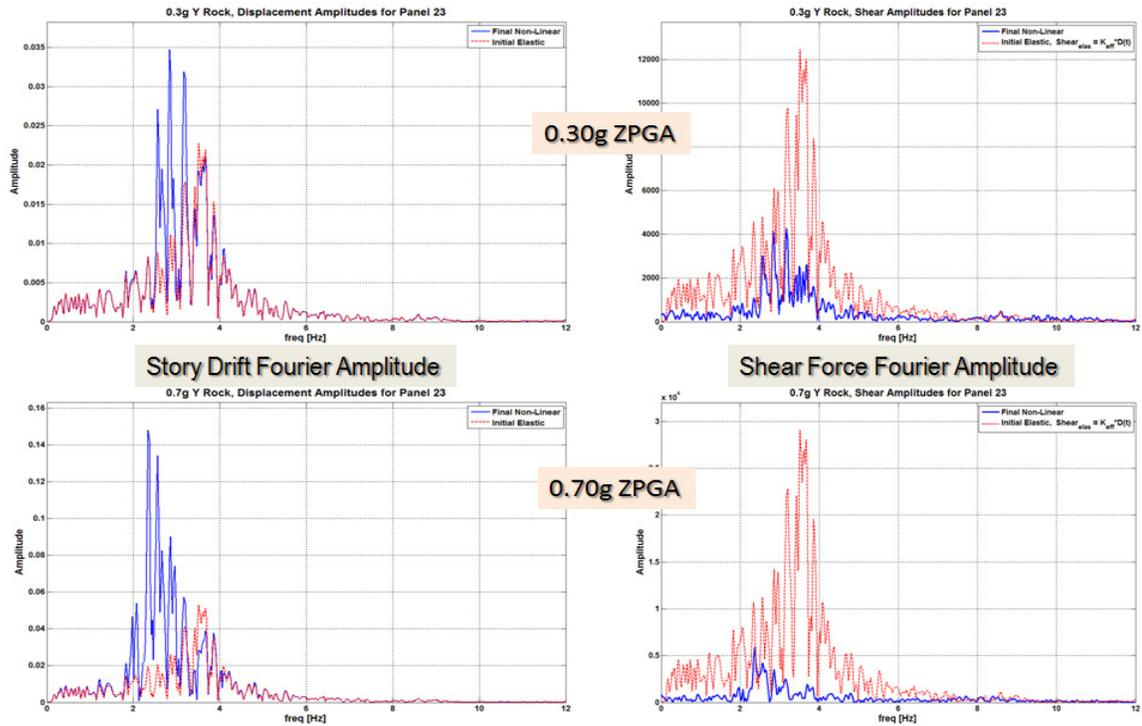
Figure 12 Linear and Nonlinear SSI Analysis Result Comparisons for Panel 23 Story Drift and Shear Force Fourier Amplitude for 0.30g and 0.70g Inputs (1<sup>st</sup> and last iterations)
