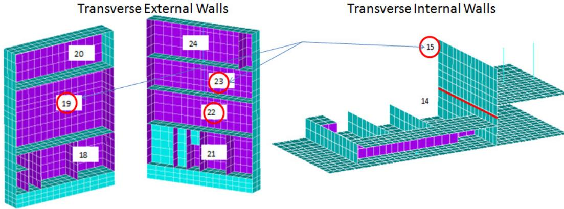
Figure 6 External and Internal Transverse Shearwall Panels
