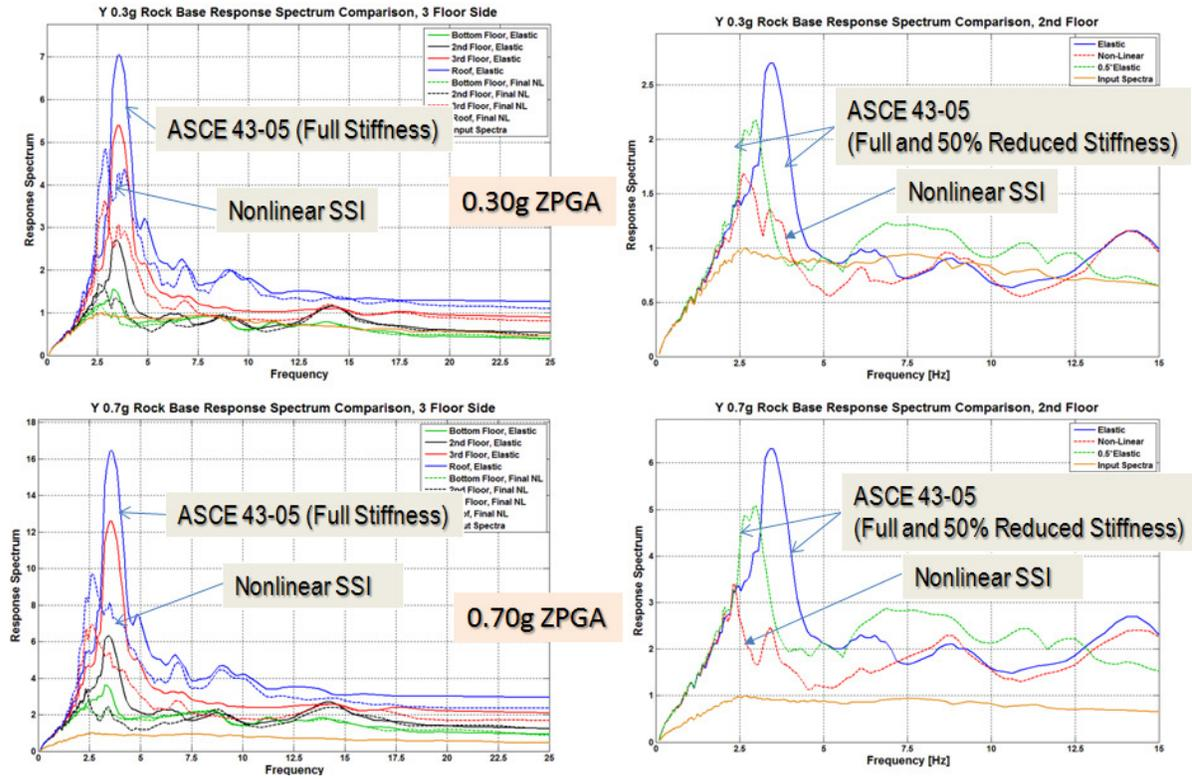
Figure 13 Linear and Nonlinear SSI Result Comparisons for 5% Damping ISRS for 0.30g and 0.70g Inputs; All Floors (left) and 2<sup>nd</sup> Floor for Both ASCE 43-05 Full and Reduced Stiffness (right)
