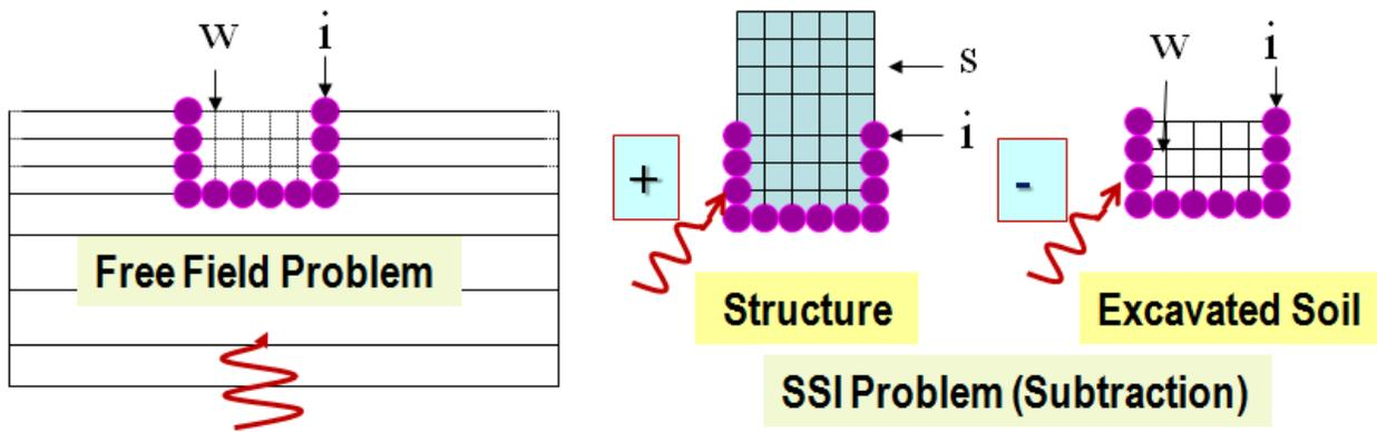
Figure 2. Subtraction Method (SM) Implementation (FI-FSIN in ACS SASSI)
