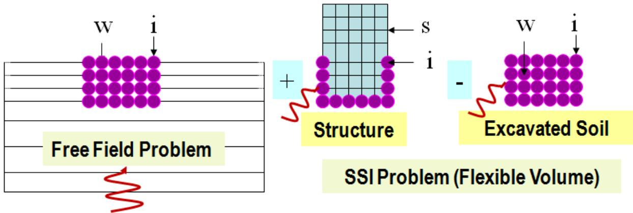
Figure 1. Flexible Volume or Direct Method (DM) Implementation (FV in ACS SASSI)
