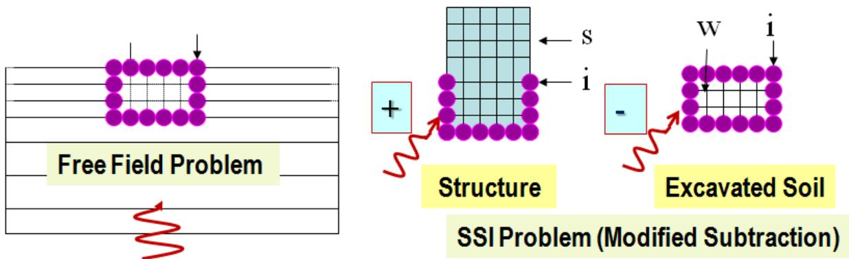
Figure 3. Modified Subtraction Method (MSM) Implementation (FI-EVBN in ACS SASSI)
