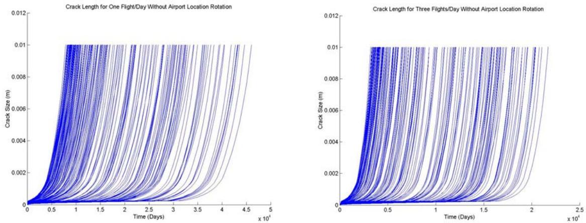
Figure 5. Simulated Crack Size Curves Without Airport Rotation
