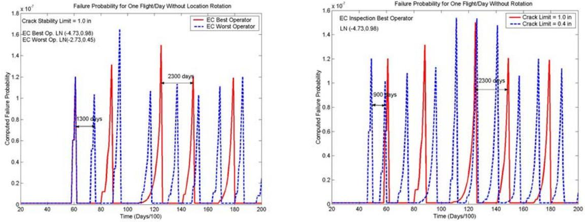
Figure 9. Risk-based Inspection Times for One-Flight/Day, Without Rotation and Given Target Risk of  $2 \times 10^{-7}$ : a) Effect of the Operator's Skill and b) Effect of Crack Limit Criterion.
