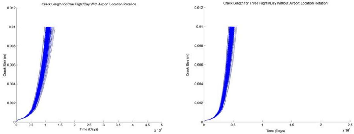
Figure 6. Simulated Crack Size Curves With Airport Rotation
