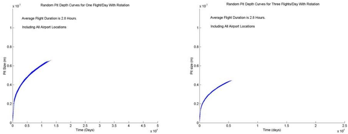
Figure 4. Simulated Pit Growth Curves With Airport Rotation
