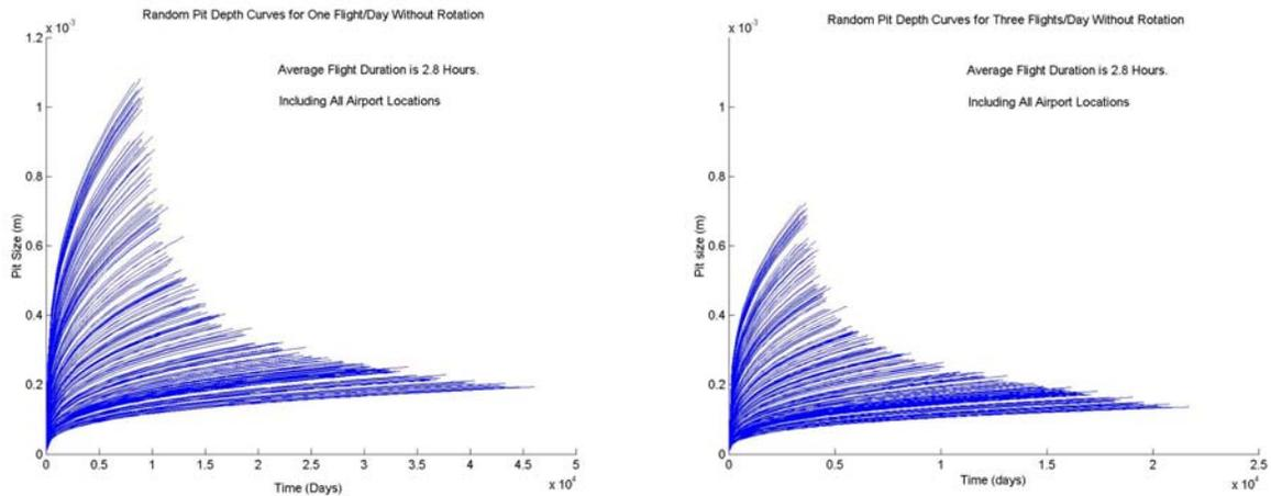
Figure 3. Simulated Pit Growth Curves for Without Airport Rotation
