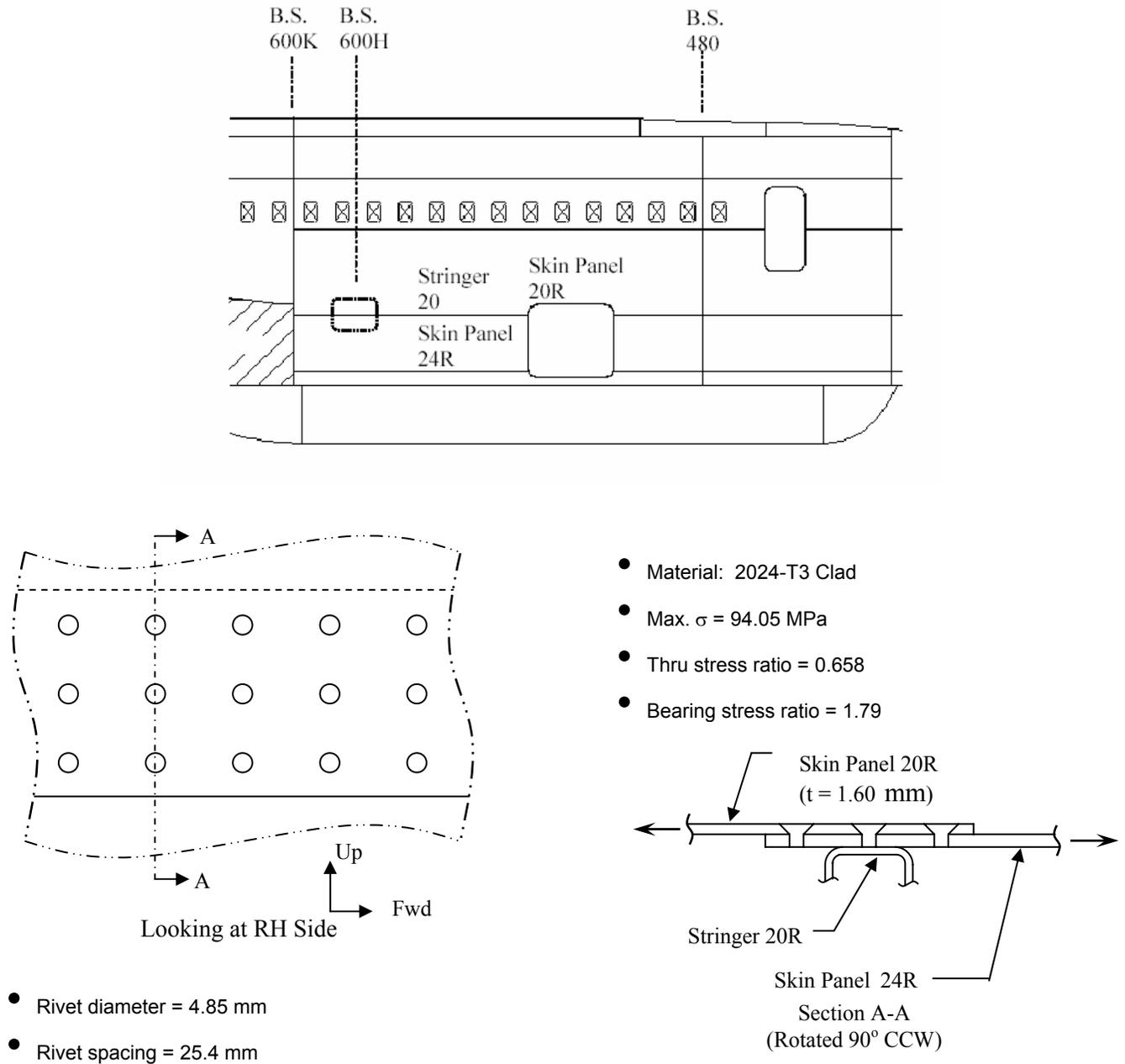
Figure 1. Details of Aircraft Structure Lap Joint
