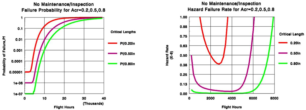
Figure 2 Failure Probability and Hazard Rate Evolution for Non-Zero Initial Condition (“Bath-Tub” shape of hazard rate curve)
