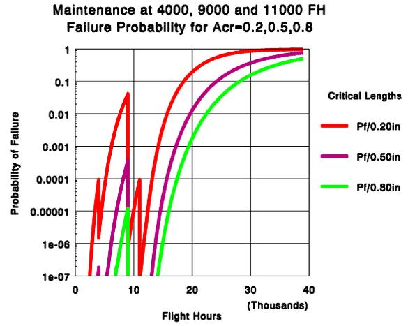
Figure 6. Failure Probability Evolution: (a) No Inspection, (b) With Inspections
