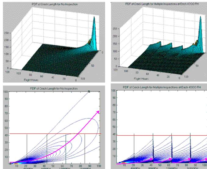
Figure 3. Effect of the NDE Inspection on Crack Length Probability Density
