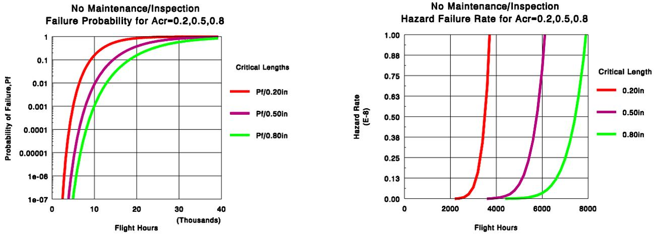
Figure 1 Failure Probability and Hazard Rate Evolution for Zero Initial Condition (“Wear-out” shape of hazard rate curve)
