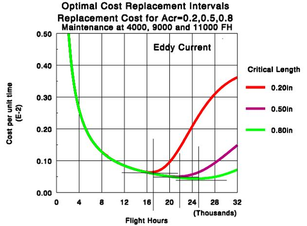
Figure 8. Maintenance Cost vs. Removal Time: (a) Visual, (b) Eddy Current
