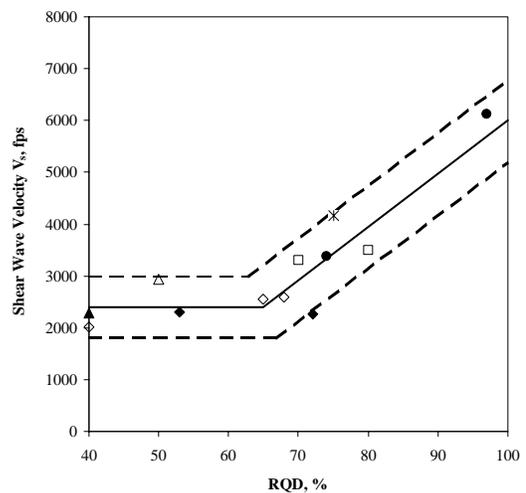
Figure 3 Measured shear wave velocities of bedrock related to the average RQD of the rock.
