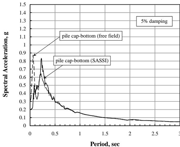
Figure 13 Comparison of the spectra at the pile cap level obtained from 3-D soil-pile analysis and free-field ground motion analysis.
