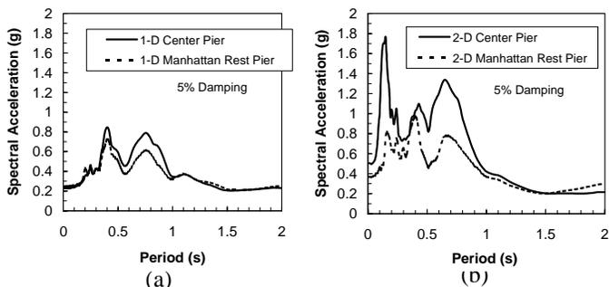
Figure 10 Comparisons of the spectra for the Center and Manhattan Rest Piers from (a) 1-D and (b) 2-D ground motion analyses.
