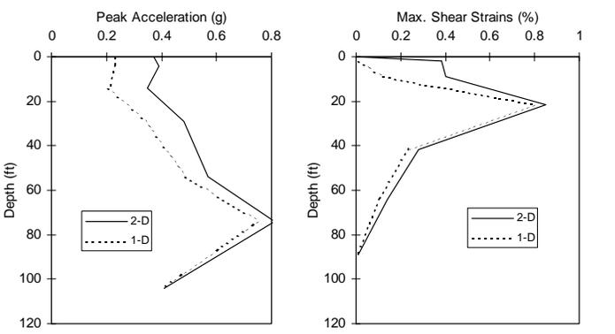
Figure 8 Comparisons of the peak accelerations and shear strains from 1-D and 2-D ground motion analyses.
