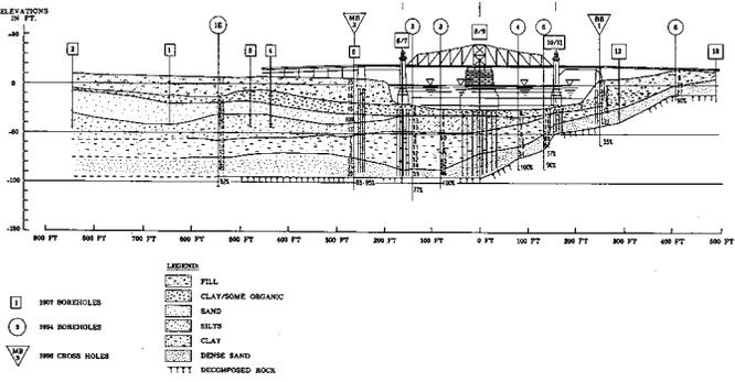
Figure 6 The soil profile and elevation of the Madison Avenue Bridge.
