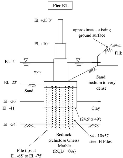
Figure 11 Elevation of Pier E1 foundation and soil profile of the Roosevelt Island Bridge.
