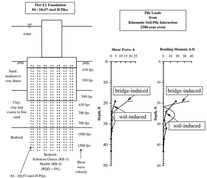
Figure 14 Pile shear forces and bending moments induced by the soil motion and bridge inertia.
