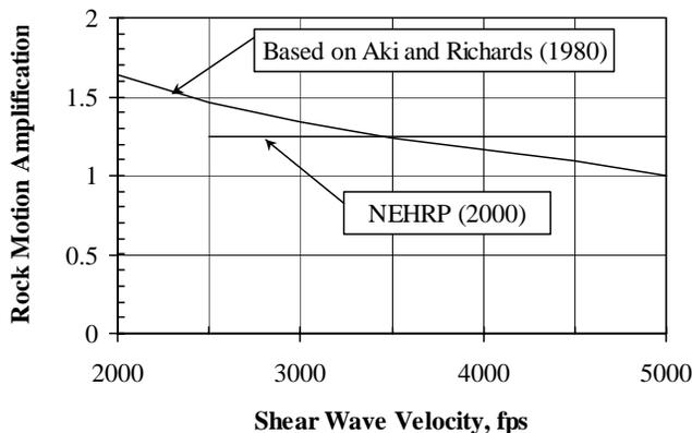
Figure 2 Rock motion amplification from hard rock ( $V_s = 5000$  fps) to softer rock.
