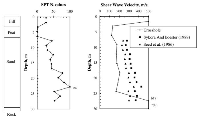
Figure 4 Comparisons of measured and estimated shear wave velocities.
