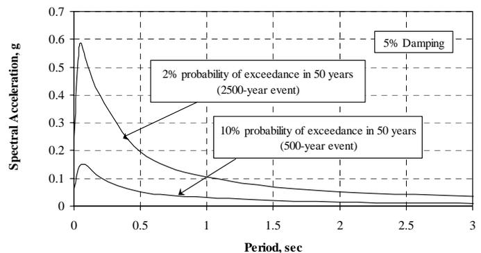
Figure 1 Hard rock spectra provided in the 1998 NYCDOT seismic guidelines. The response spectra shown, in effect, define the seismic design level input at outcropping of hard rock. These spectra were
