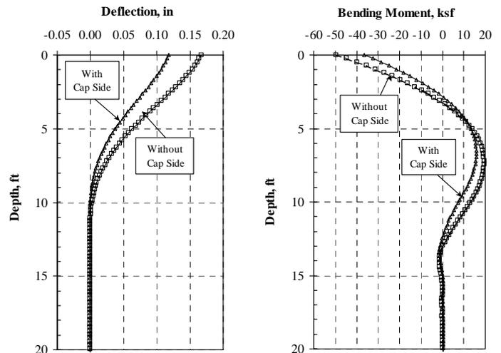
Figure 17 The effect of including pile cap side resistance on the pile deflections and bending moments.
