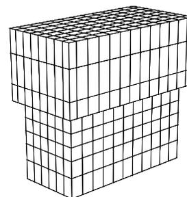
Figure 12 Three-dimensional model of soil-pile system of Pier E1 used in SASSI analysis.
