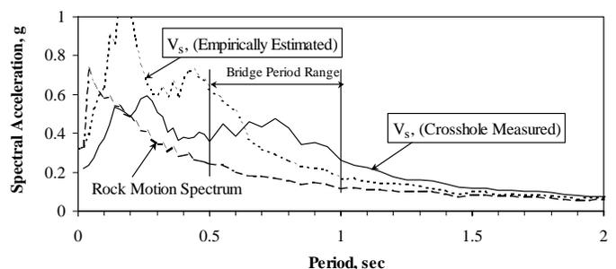
Figure 5 Comparison of the response spectra from ground motion analyses, using the crosshole measured, and empirically-estimated shear wave velocities. This motion was subsequently used as input in the seismic analysis of the bridge.
