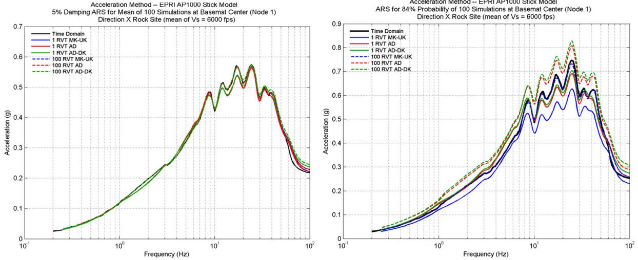
a) Basemat Center, X Direction – Rock Site – Mean ISRS (left) and 84% Probability ISRS (right)
