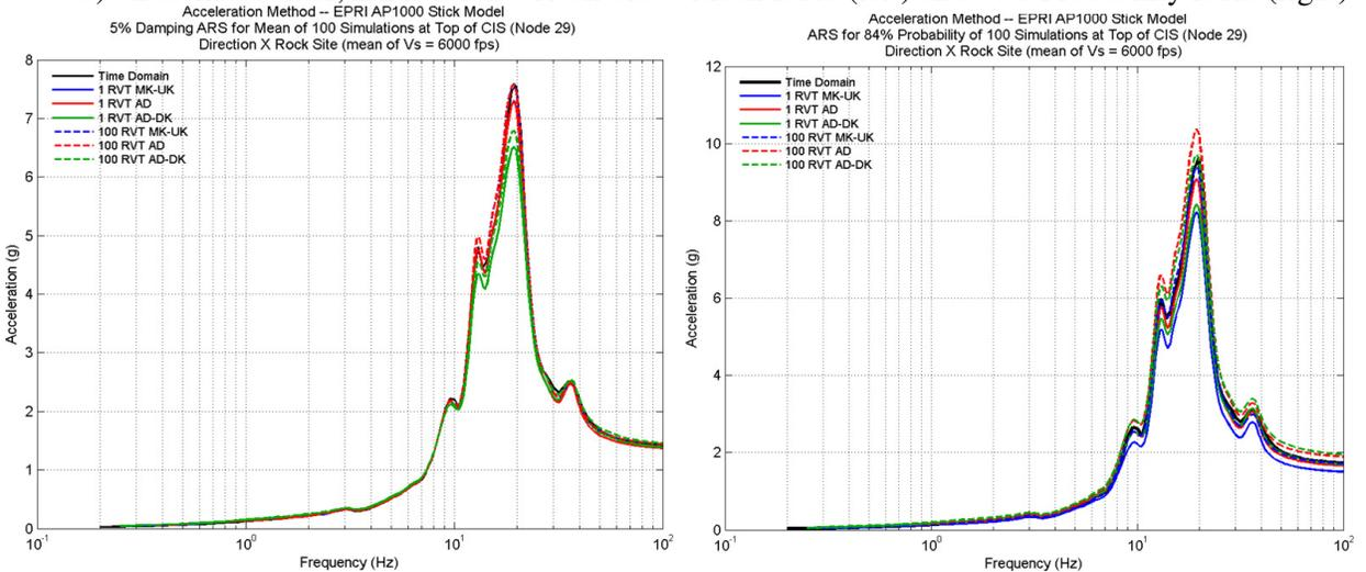
c) Top of CIS, X Direction – Rock Site – Mean ISRS (left) and 84% Probability ISRS (right)
