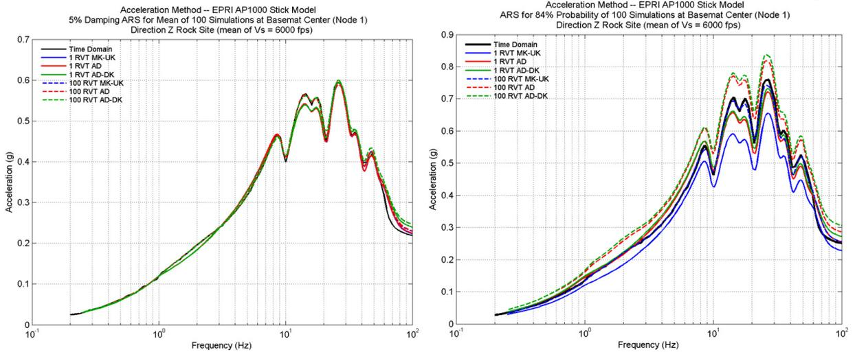
b) Basemat Center, Z Direction – Rock Site – Mean ISRS (left) and 84% Probability ISRS (right)
