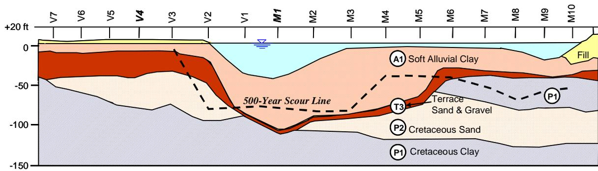
Figure 2. Soil profile and bridge pier locations.
