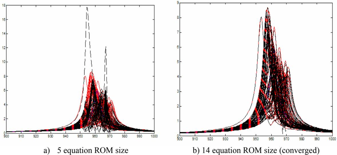
Figure 5. Computed blade tip amplitudes using the full-analysis model and the SPM ROM approach, with a 5 equation ROM size or 5 basis vectors, and a 14 equation ROM size or 14 basis vectors, respectively. Modified Blisk Design (red solid line is the full-analysis, black dashed line is the SPM ROM).
