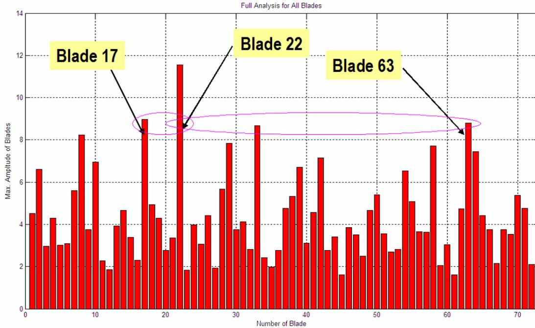
Figure 6. Simulated mistuned blade tip amplitude pattern for the 72 blade blisk system
