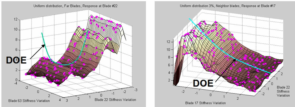
Figure 7. Response surfaces of the blade tip amplitudes for blades 22 as a function of stiffness variation of blade pair 22 and 63, and 22 and 17, respectively (see Figure 6).
