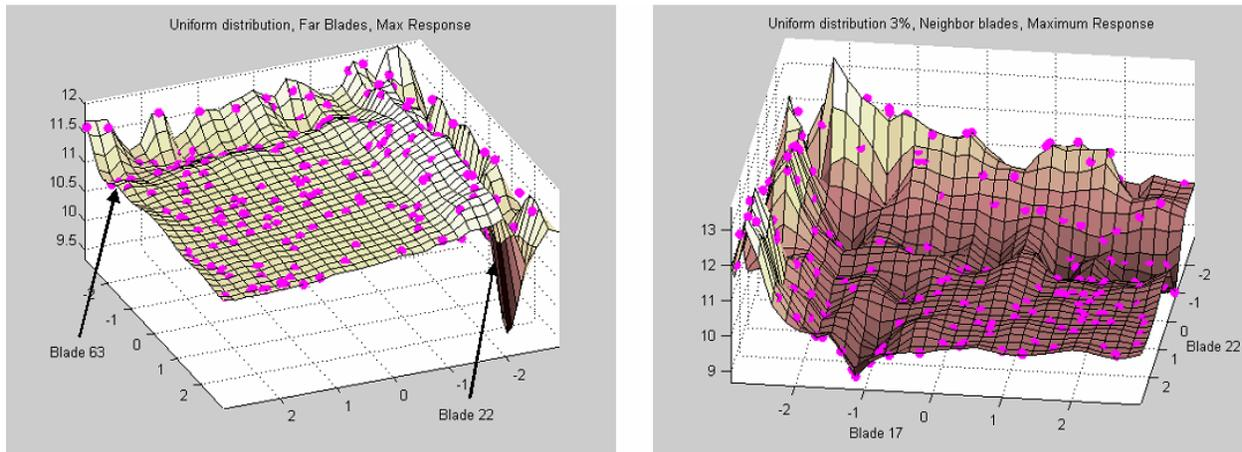
Figure 8. Response surfaces of the maximum blade tip amplitude around the blisk wheel as a function of the stiffness variation of the blades of the pairs 22 and 63, and 22 and 17, respectively (see Figure 6)
