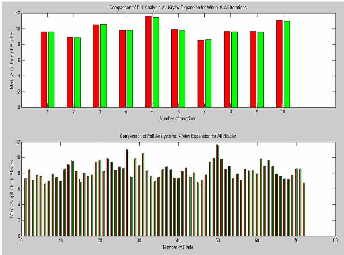
Figure 2. Blade tip responses, per simulation (upper plot) and per blade location (lower plot), computed using full-model analysis (red) and SPM ROM approach (green) for ten realizations of stochastic input
