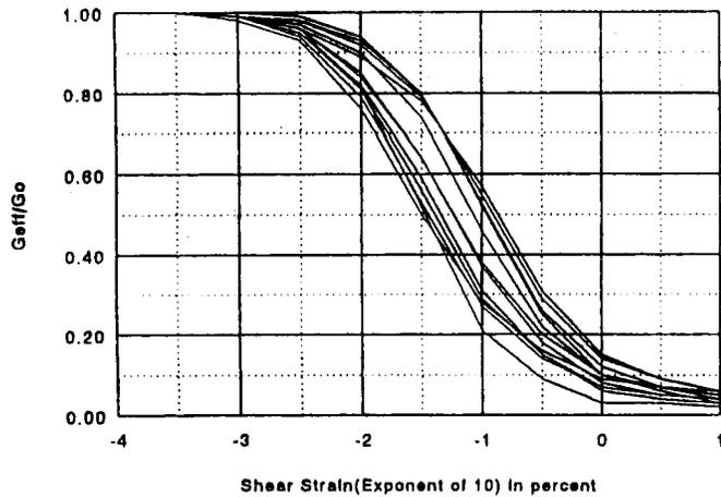
**Fig. 8.** Realizations of shear modulus versus shear strain curve
