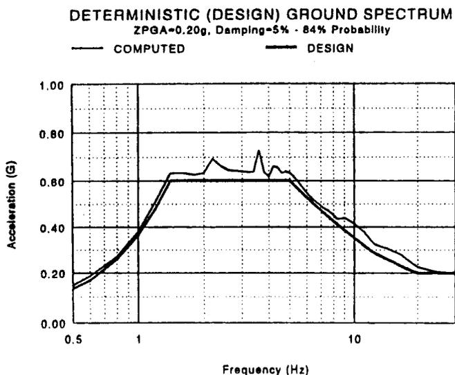
**Fig. 3.** Computed versus design ground response spectra
