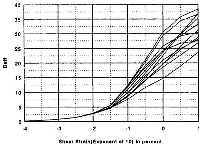
**Fig. 9.** Realizations of damping versus shear strain curve
