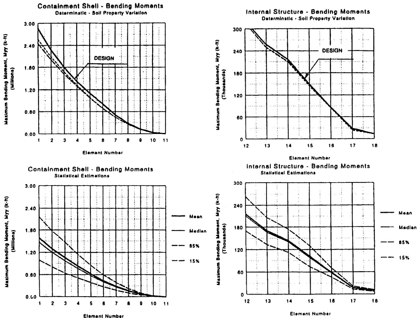
Fig. 11. Comparison of deterministic and probabilistic bending moment in reactor building structure
