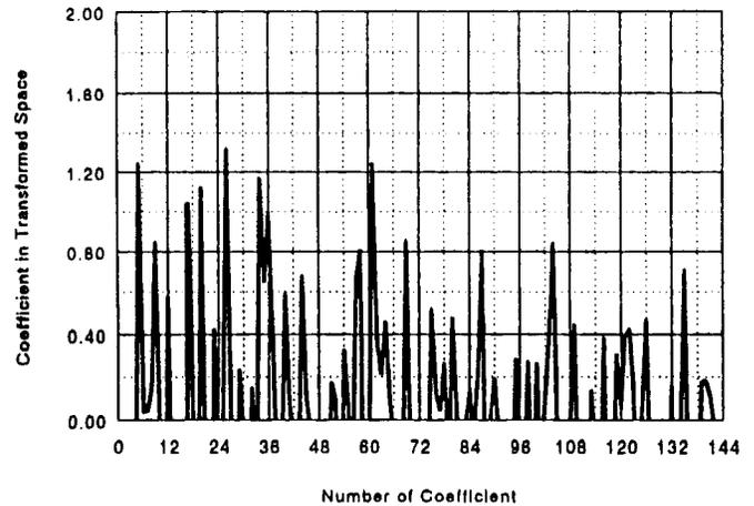
**Fig. 10.** Coefficient of polynomial chaos expansion of the stochastic base bending moment solution
