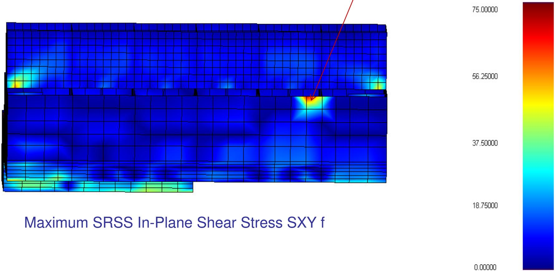
Maximum SRSS In-Plane Shear Stress SXY f
