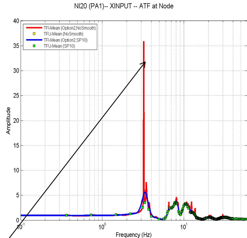
“Spurious” ATF Peak Produced by the Interpolation Function
