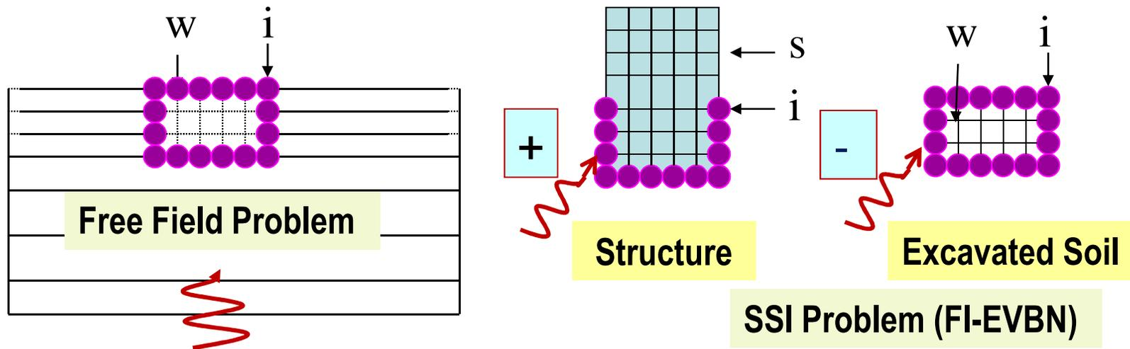
**Flexible Volume Method** (the interaction nodes are all excavated volume nodes, w and i)
