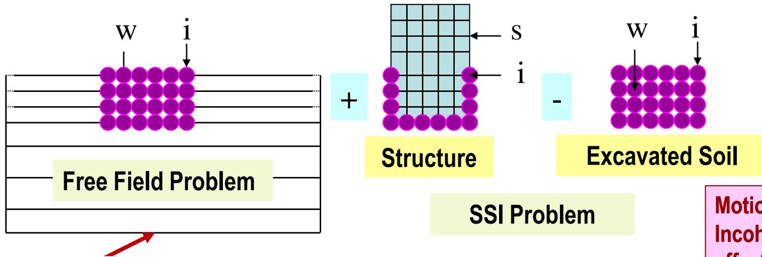
**Flexible Volume Method** (using all excavated volume nodes)
