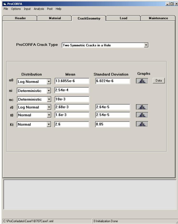
Figure 3-7 Crack Geometry Model
