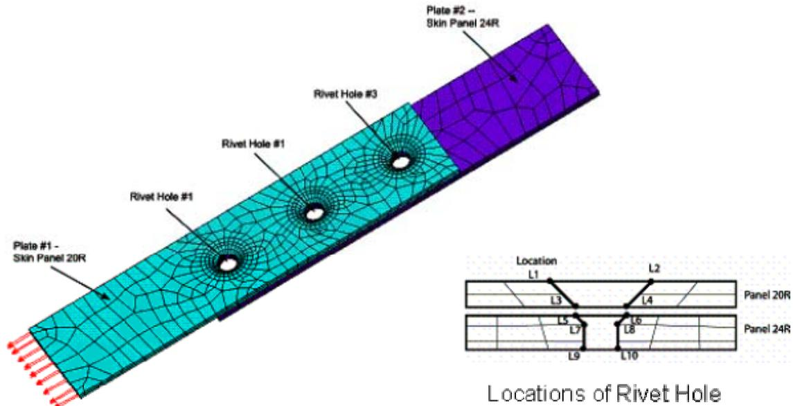
**Figure 2-2 B707 Critical Stress Locations in the lap joint**
