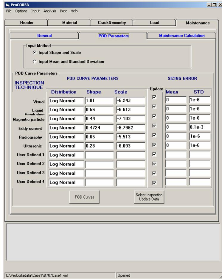
Figure 3-10 POD Parameters
