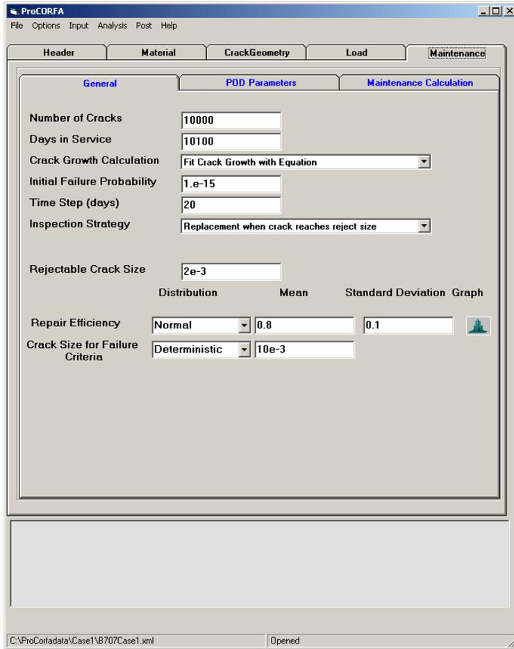
Figure 3-9 Maintenance General Parameters
