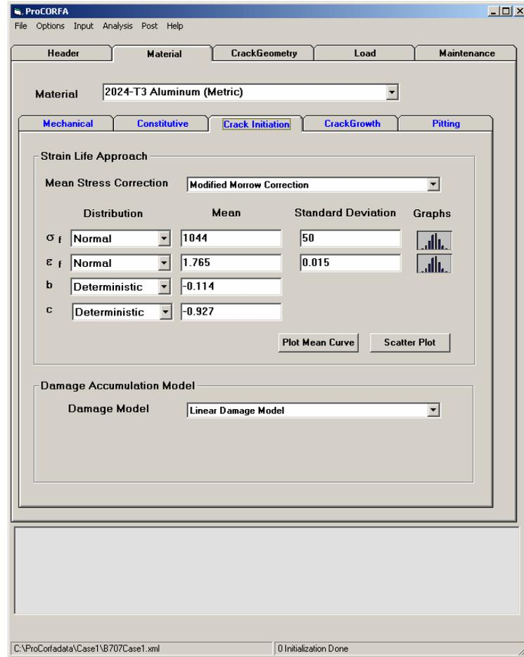
Figure 3-4 Crack Initiation Model
