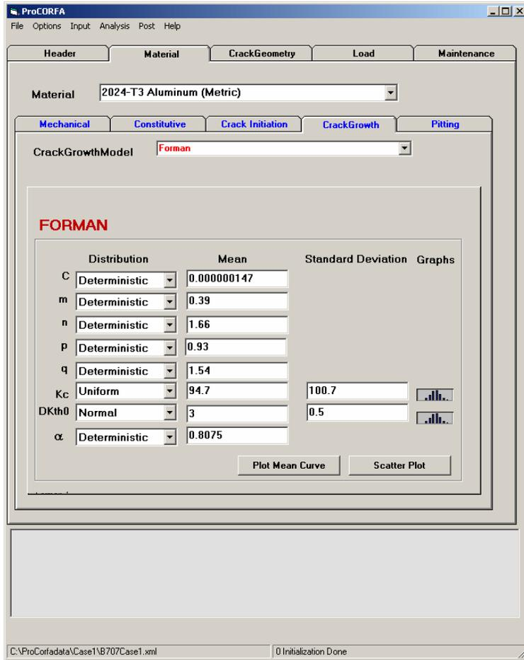
Figure 3-5 Crack Growth Model
