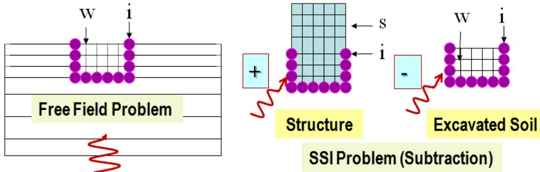
Figure 2. Subtraction Method (SM) Implementation
